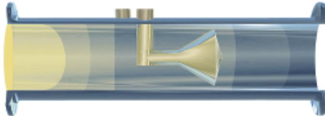
*As the flow approaches the cone, the flow profile “flattens” toward the shape of a well developed profile—even in extreme flow conditions.*
