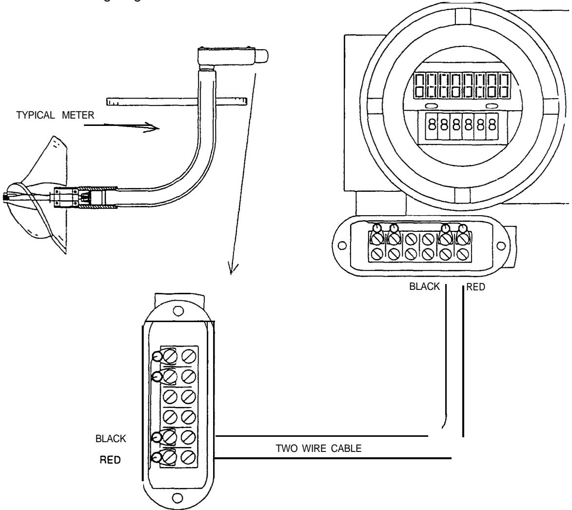
The positions of the wires in the condulets is not important. The black wires should be connected together, and the red wires should be connected together.
