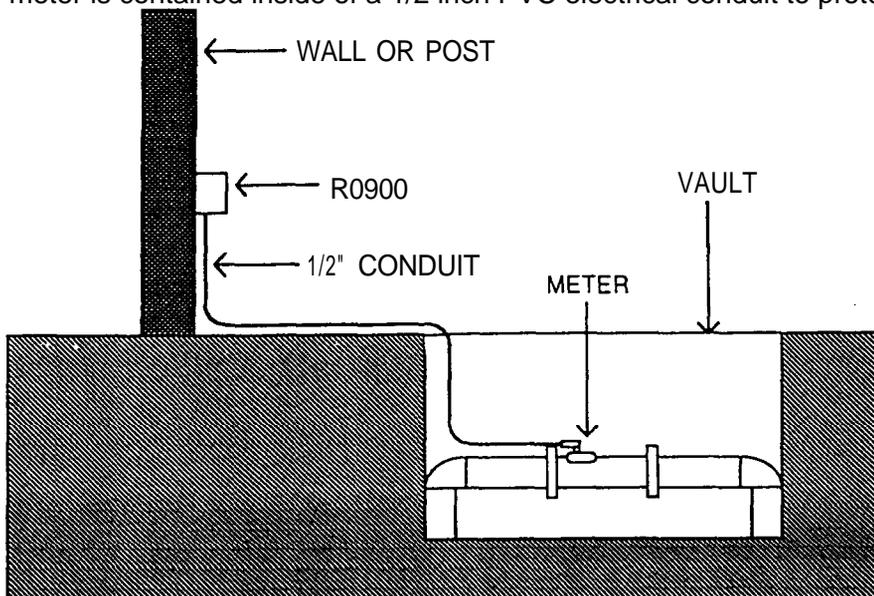
The electrical conduit must be sealed from any moisture by using silicone sealer to protect the electronics. Therefore it is recommended that threaded connectors be sealed with Teflon sealing tape and the PVC conduit be glued. It is also recommended that the R0900 be mounted facing north or in a shaded area to avoid sun damage to the LCD.
